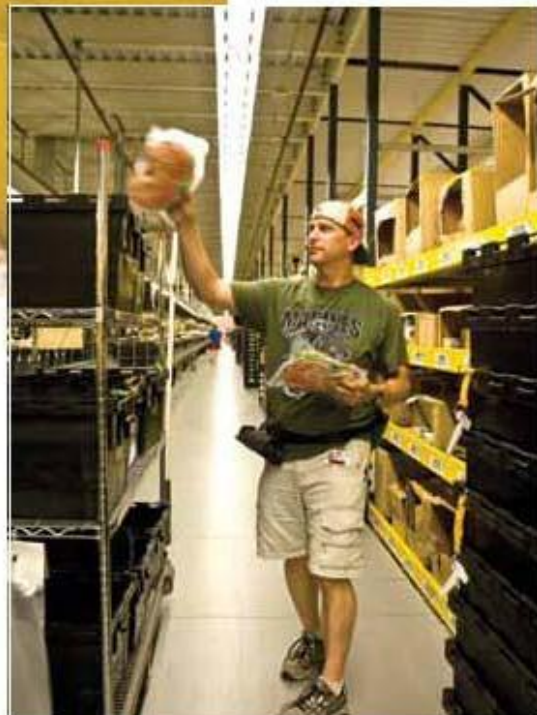
Oriental Trading's WCS creates a wave of 100,000 items to fill 10,000 orders. Once picked (bottom right), orders are assembled by a tilt tray sortation systems which routes the required items to a packing station (top left) where associates pack orders for delivery.
