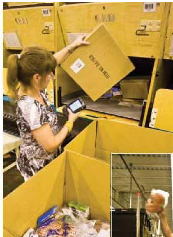
Oriental Trading's WCS creates a wave of 100,000 items to fill 10,000 orders. Once picked (bottom right), orders are assembled by a tilt tray sortation systems which routes the required items to a packing station (top left) where associates pack orders for delivery.
